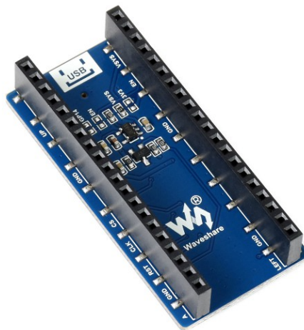
Figure 23: Underside View of 1.14 LCD Display. This view shows the Pico attachment sockets and how the pins used by the display are labeled [18]. We had to figure out a way to preserve this attachment method with our own board between the two devices, and the solution was to use double-sided headers with a socket for the Pico and pins on the other side for the display.
