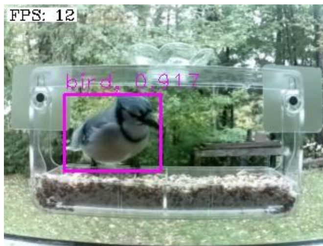
Figure 9: Final Frame of Bird including FPS, Box, Label, and Confidence Score
