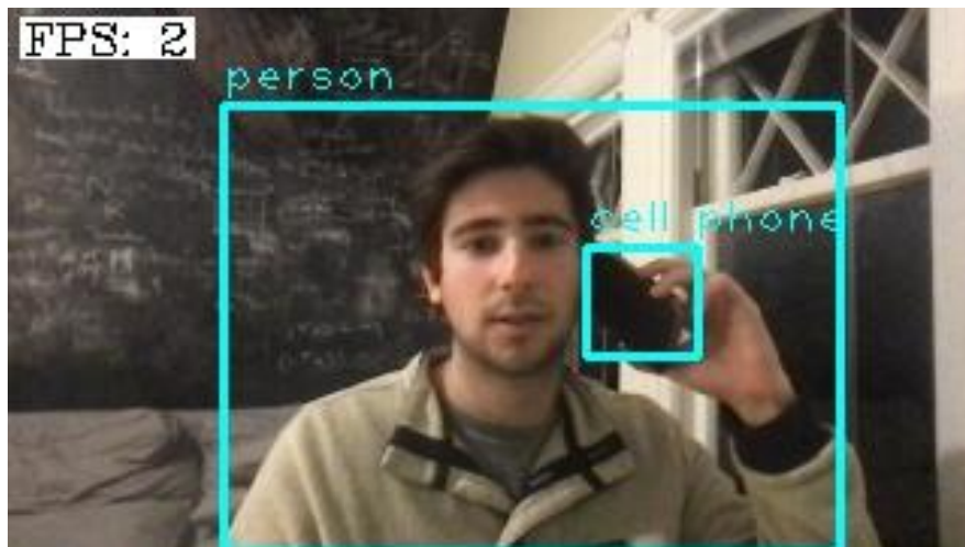
Figure 11: Correctly Identifying Multiple Objects at the Same Time is Very Slow (2 FPS)
