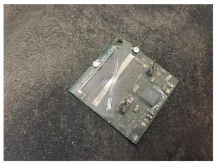
Fig. 6 Impact test article on bed of lunar regolith simulant after exposure to 27,000g of acceleration to simulate impact with the lunar surface.
