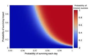
Fig. 8 Probability of mission success, defined as 5 of 100 chipsats surviving on the surface of a celestial body for 100 days, for a range of impact survival probabilities and daily survival probabilities.
