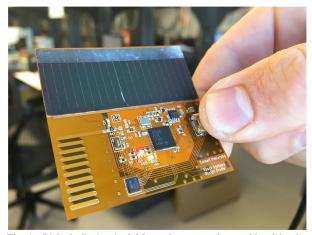
Fig. 1 Biologically inspired Monarch spacecraft, capable of in situ sensing and radio networking with other Monarchs and with ground-based receiver stations.
