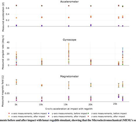
Fig. 7 IMU measurements before and after impact with lunar regolith simulant, showing that the Microelectromechanical (MEM)'s sensor survives and continues to operate to within the specifications of the datasheet [34].
