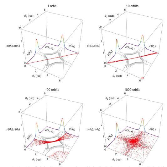
Fig. 5 True anomalies of two Monarchs deployed on orbits at geostationary altitude and inclination after varying numbers of orbits. Orbits are identical, except a variation in eccentricity by one-tenth of a percent.
